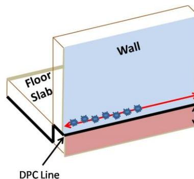
Drill Holes are spaced 100mm apart. Drilling & Injection will be done 1-brick height above the DPC line i.e on the red line in the diagram.
